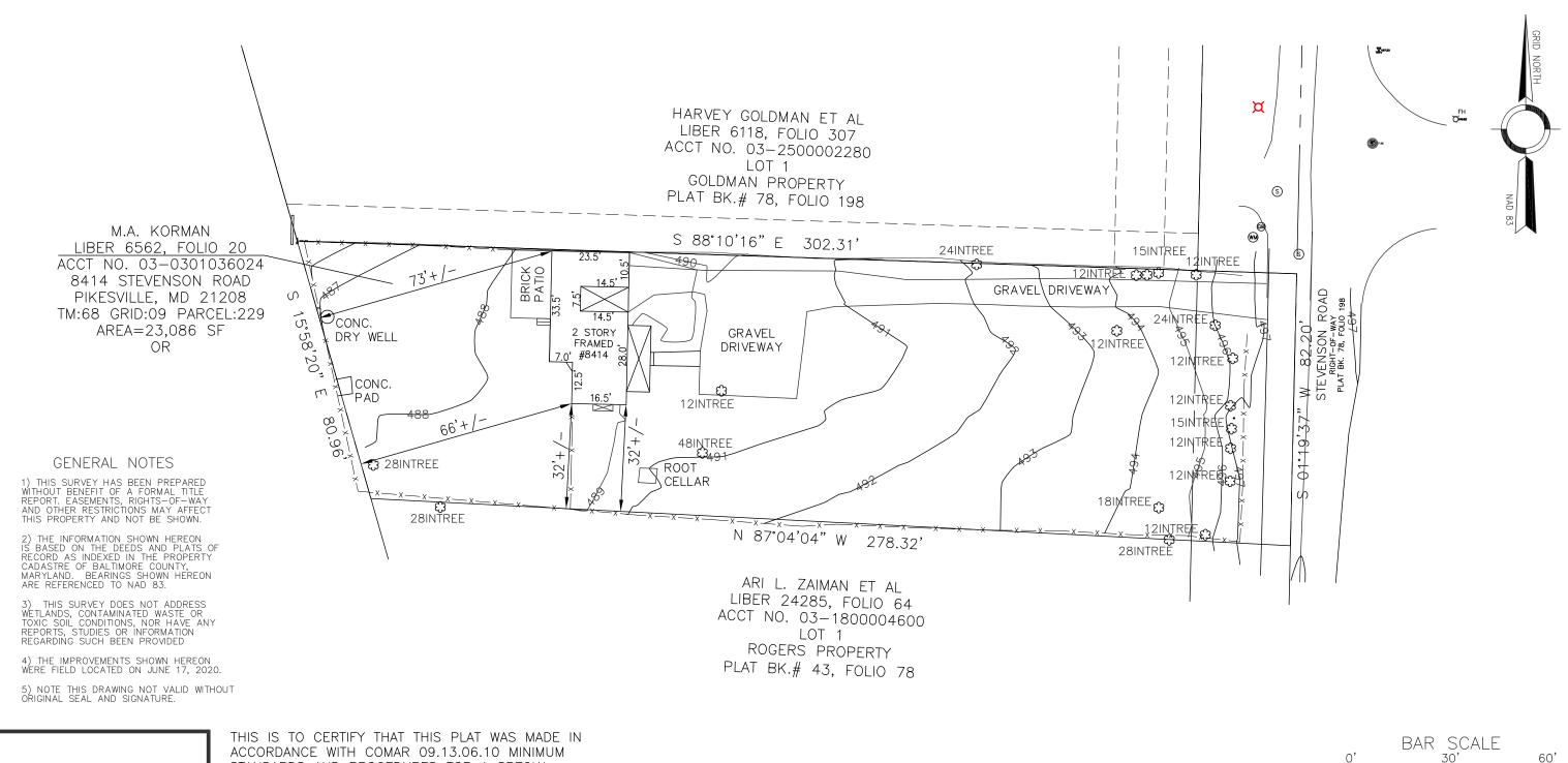
THIS IS TO CERTIFY THAT THIS PLAT WAS MADE IN ACCORDANCE WITH COMAR 09.13.06.10 MINIMUM STANDARDS AND PROCEDURES FOR A SPECIAL PURPOSE SURVEY. THE VISIBLE IMPROVEMENTS ARE SHOWN TO A TOLERANCE OF 1 FOOT MORE OR LESS.
